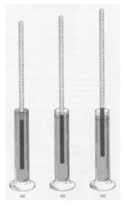
Figure 2: Measuring the volume of gas at room pressure.
